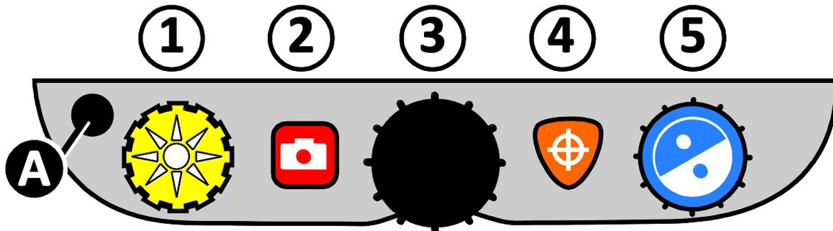
The black **ADVANCED** button (**A**) is used with other control panel buttons and dials to access and perform more features and operations.
